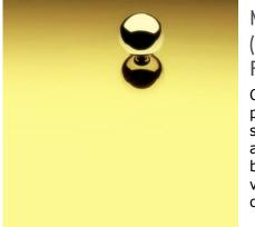
No. 8 Finish (Mirror Polished) Obtained by polishing with successively finer abrasives, then buffing with a v e r y f i n e compound.
